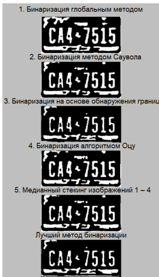
Fig. 2. Number plates binarized by various methods
