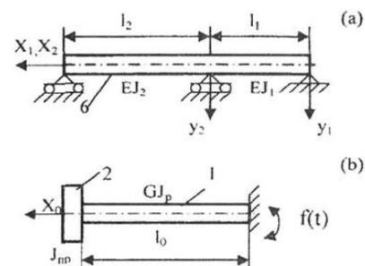
Fig. 3. Dynamic model (idle rail)
