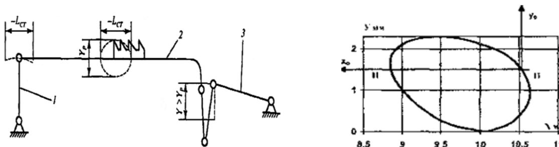
Fig. 1. Kinematic diagram of the mechanism and the trajectory of the rack
