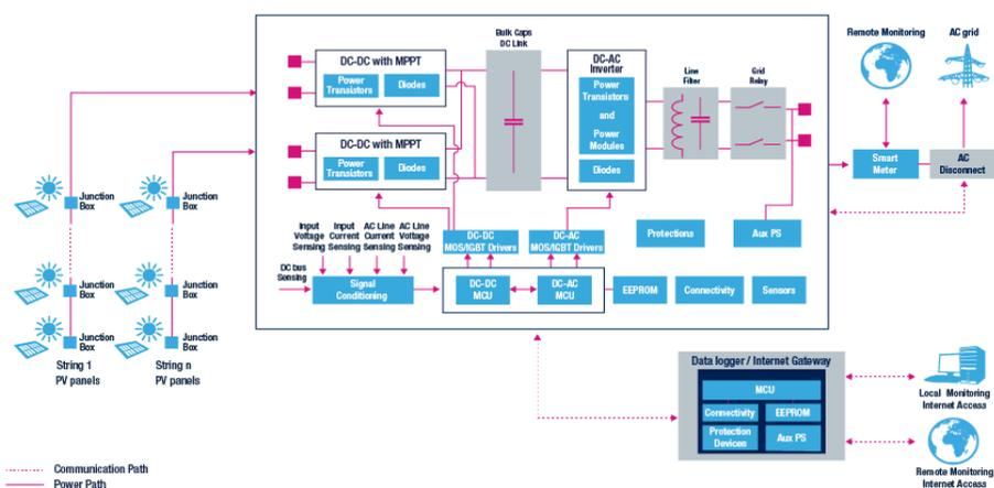
**Fig. 8 Functional diagram of a solar PV generation system using a central PV inverter and PV strings**
