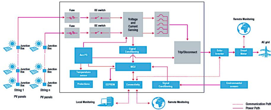
**Fig. 7 Functional diagram of a solar PV power generation system using a smart string combiner box**
