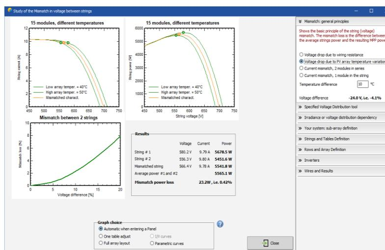
**Fig. 1 Panel of results of calculated generation characteristics of PV module produced by AE Solar, type AE400DGLM6-72(1500), 15 modules connected in series**
