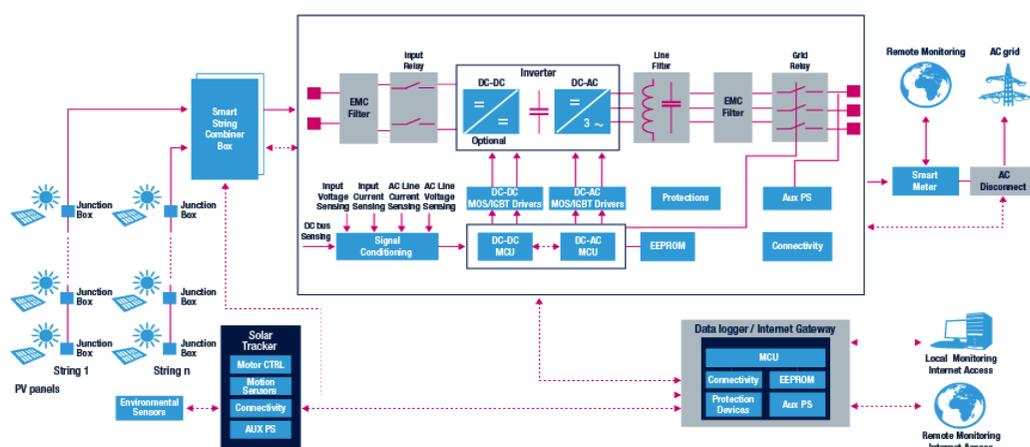
Fig. 6 Main functional components of PV electric generation systems
