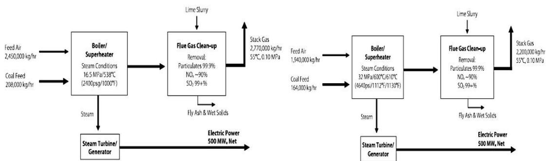
**Fig. 1 Functional diagrams of a coal-fired thermal power plant without CO<sub>2</sub> capture using "subcritical" technology (left) and "ultra-supercritical" technology (right)**
