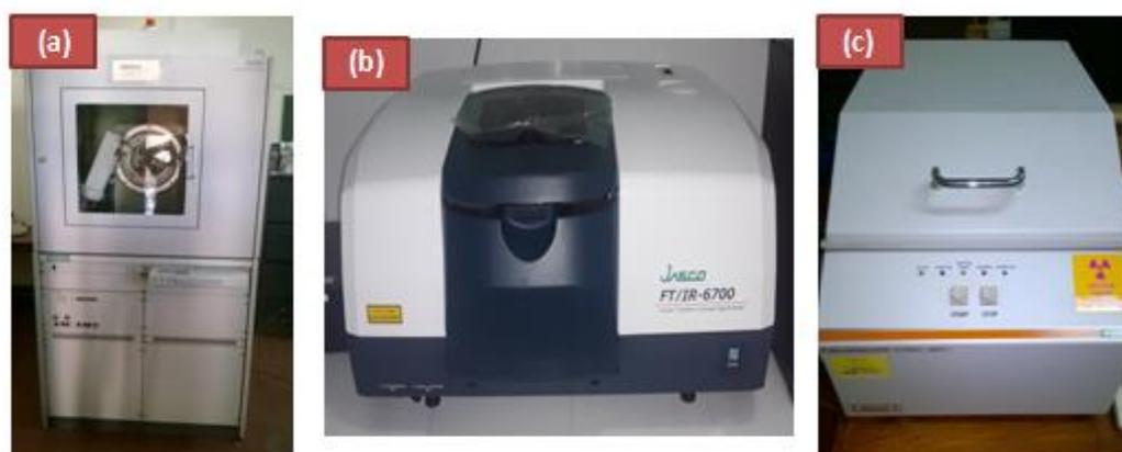
Fig. 4. (a) X-ray diffraction (XRD) spectrometer, (b) Fourier transforms infrared (FT-IR) spectrometer and (c) X-ray fluorescence (XRF) spectrometer
