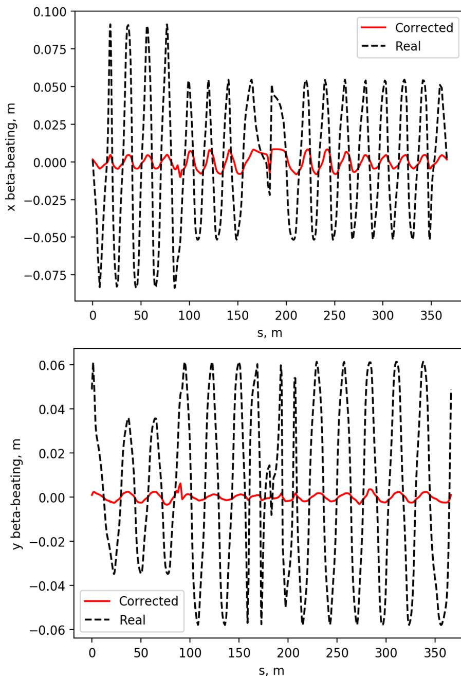
**Fig. 2. Horizontal (upper) and vertical (lower) betatron functions before and after correction**
