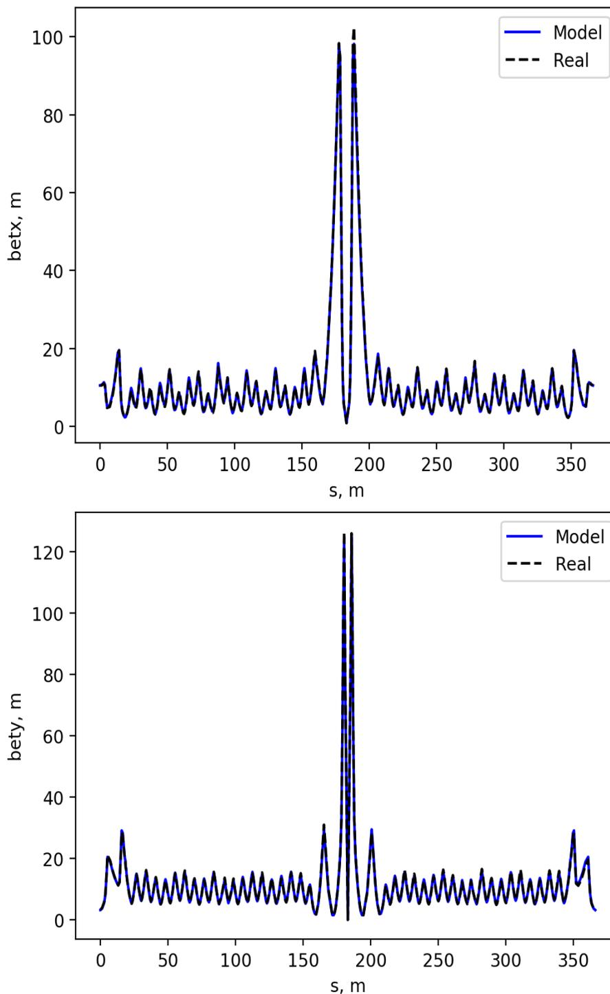
Fig. 1. Horizontal (upper) and vertical (lower) betatron functions
