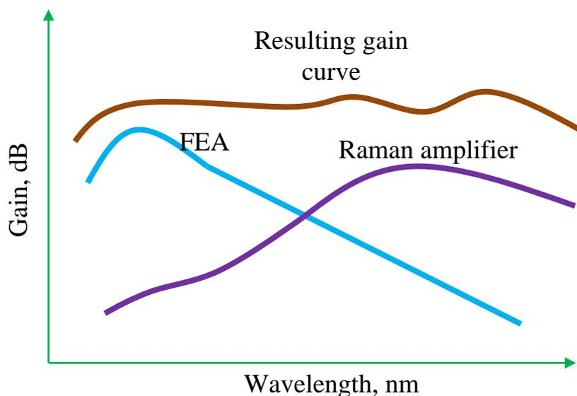
**Fig. 2. Smoothing the overall gain curve when using stimulated Raman scattering - amplifier and erbium fiber amplifier**
