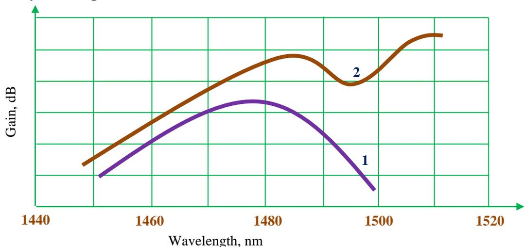
**Fig. 1. Spectral curves of stimulated Raman amplification - amplifier pumped at one (1) and two (2) wavelengths**
